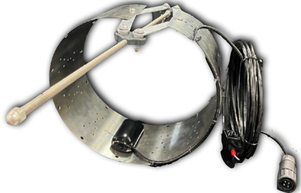
Single AV Sensor with Band and Screw-Jack
