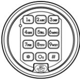
**Step 1**—Remove the battery tray from underneath the bottom of the keypad. Catch the small notch and pull the housing slightly toward the front of the keypad. Slide tray down and pull out and remove old battery.
