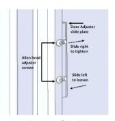
should feel slight resistance when turning the handle to extend the door bolts. Only slight movement should be felt with the door is shut. Caution: Do not adjust door too tight. This may cause wear on both the door pins and locking mechanism. If your door has a tendency to self-open (the bolts retract by themselves) or the handle is hard to turn when extending the bolts, the door adjusters may be too tight.
