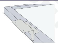
2 Place each of the mounts 30-40 cm in from the end, on the long side. Place the smallest face of the Z-Bracket on the panel with the legs of the bracket pointing towards the glass side.
