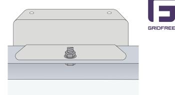
4 Attach the Z-bracket to the solar panel. Put the bolt through from the underside then put the large washer over it, followed by the spring washer, then tighten the nut down firmly.
