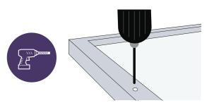
3 Mark inside the hole of the Z-Bracket, then remove the bracket and drill a 6mm hole on the underlip of the panel. Be careful to only drill through the panel frame.
