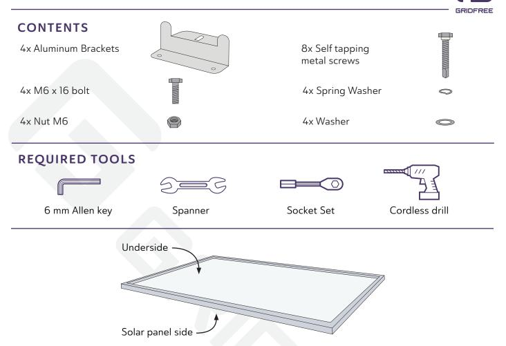
1 When installing the Z–Brackets, have the solar panel upside down so the underside is facing you. Lay it on cardboard or another soft surface to avoid scratching the glass.
