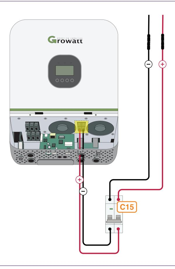
Run the excess 6mm² positive(+) and negative(-) cables from the C15 circuit breaker to the hybrid inverter.
