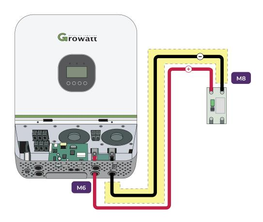
Wire the negative(-) 35mm<sup>2</sup> M6+M8 cable from the hybrid inverter to the 125A MCCB circuit breaker.
