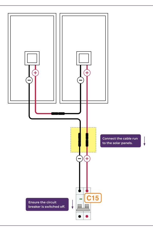
When the cables have been terminated in the circuit breaker and the circuit breaker is switched off, you can now connect the solar panels to the cable run. The circuit breaker must be switched off when connecting or disconnecting the solar panels from the cable run.
