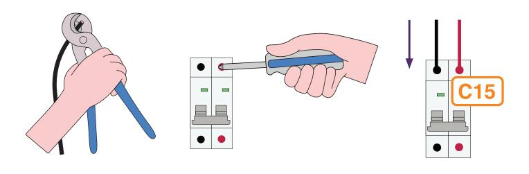
Use wire strippers to strip the ends of the solar cable, and terminate them in the circuit breaker by inserting the stripped end and tightening the screw clockwise. Make sure the clamp inside the circuit breaker is in contact with the metal conductor, and **NOT** the insulation of the wire.
