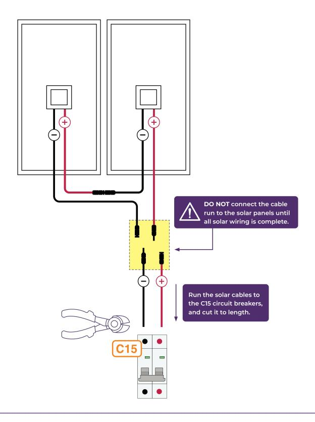
2 Run the 6mm<sup>2</sup> PV solar cables from the solar panels back to the C15 circuit breakers, and cut it to length.
