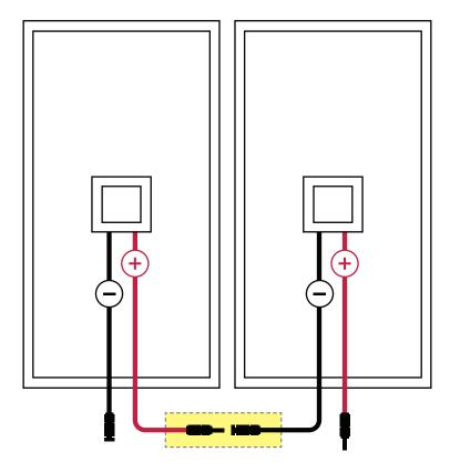
Wire the panels together by connecting the positive terminal of one panel to the negative terminal of another. This creates two solar array outputs: one positive, one negative (-).
