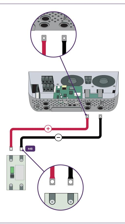
Before proceeding to connect the hybrid inverter to the 125A MCCB circuit breaker, align the 35mm<sup>2</sup> x 1m cables between the components to ensure that the M6 ends (smaller holes) are inserted into the hyrbid inverter, and the M8 ends (larger holes) are inserted into the circuit breaker.
