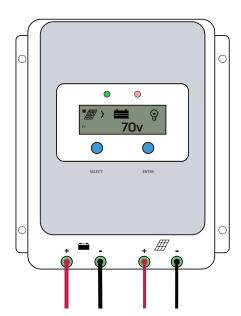
The Green LED on the charge controller should flash, and the panel voltage should be around 60-70V in full sunlight. As this charge controller auto-detects voltage, on its first start up it can sometimes default to 12V, and will give a battery over voltage warning.
