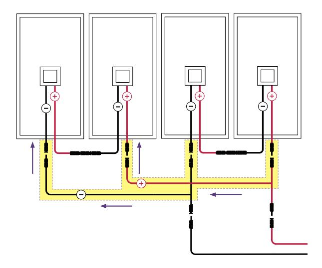
3 Connect the other pair of solar panels to the Y-branch connectors, connecting the negative terminals from each pair with the black Y-branch connector, and the positive terminals from each pair with the red.
