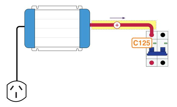
Wire the positive (+) 25mm cable from the inverter to the Cl25 circuit breaker.
