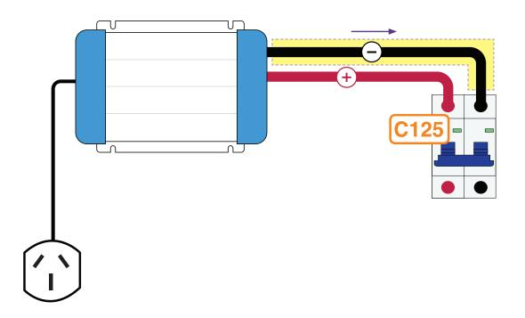
11 Wire the negative (-) 25mm cable from the inverter to the Cl25 circuit breaker.
