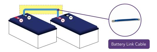
The battery bank is wired with two 12V batteries in series, this creates a 24V battery bank. The large gauge cable is used to connect the batteries together and used to connect to the inverter.
