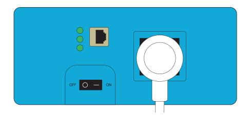
Flick the "ON" switch located on the side of the inverter, and check that all three LED indicators show green. If any do not show green, consult the inverter manual to identify the fault.
