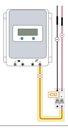
7 Wire the positive (+) 6mm cable from the charge controller to the C32 circuit breaker.
