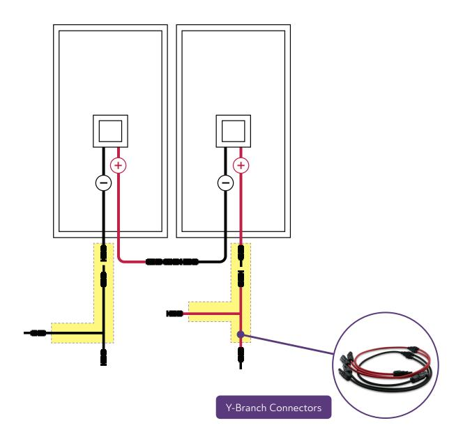
2 Connect the Y-branch connectors to one of the solar panel pairs.
