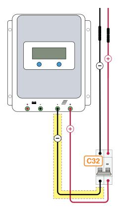
8 Wire the negative (-) 6mm cable from the charge controller to the C32 circuit breaker.
