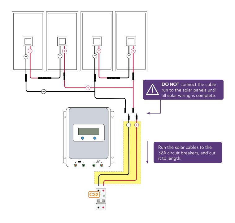
Run the 6mm solar cables from the solar panels back to the 32A circuit breakers, and cut it to length.
