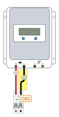
Wire the negative (-) 16mm cable from the charge controller to C63 circuit breaker.
