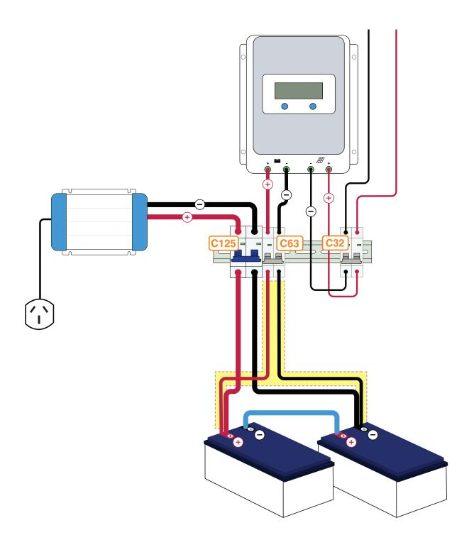
Wire the remaining set of red and black 16mm cable to the charge controller through the C63 circuit breaker.
