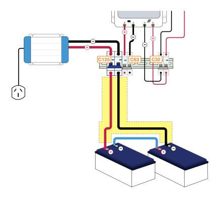
15 Wire the remaining set of red and black 25mm cable to the inverter through the Cl25 circuit breaker.
