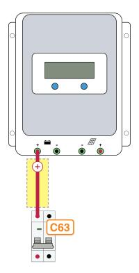
Wire the positive (+) 16mm cable from the charge controller to C63 circuit breaker.
