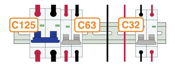
Switch on the circuit breakers in the following order. First switch on the battery to charge controller breaker C63. Then the battery to inverter C125. Finally, the panels to the charge controller C32.
