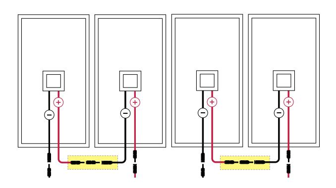
Start by creating two pairs of panels wired together. Connect the positive terminal of one panel to the inline fuse, then to the negative terminal of the next panel.
