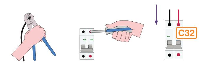
Use wire strippers to strip the ends of the solar cable, and terminate them in the circuit breaker by inserting the stripped end and tightening the screw clockwise. Make sure the clamp inside the circuit breaker is contacting the metal conductor, and **NOT** the insulation of the wire.
