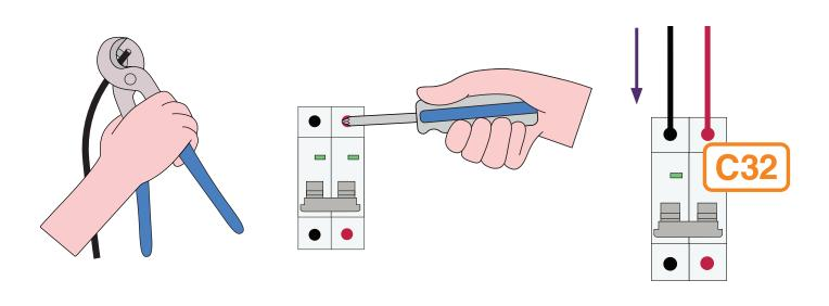
Use wire strippers to strip the ends of the solar cable, and terminate them in the circuit breaker by inserting the stripped end and tightening the screw clockwise. Make sure the clamp inside the circuit breaker is in contact with the metal conductor, and **NOT** the insulation of the wire.
