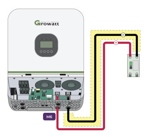
Wire the negative(-) 35mm<sup>2</sup> M6+M8 cable from the hybrid inverter to the 125A MCCB circuit breaker.
