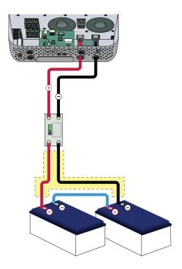
Wire the 35mm<sup>2</sup> 3m set of red and black cables to the inverter through the 125A MCCB.
