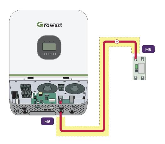
Wire the positive(+) 35mm<sup>2</sup> M6+M8 cable from the hybrid inverter to the 125A MCCB circuit breaker.
