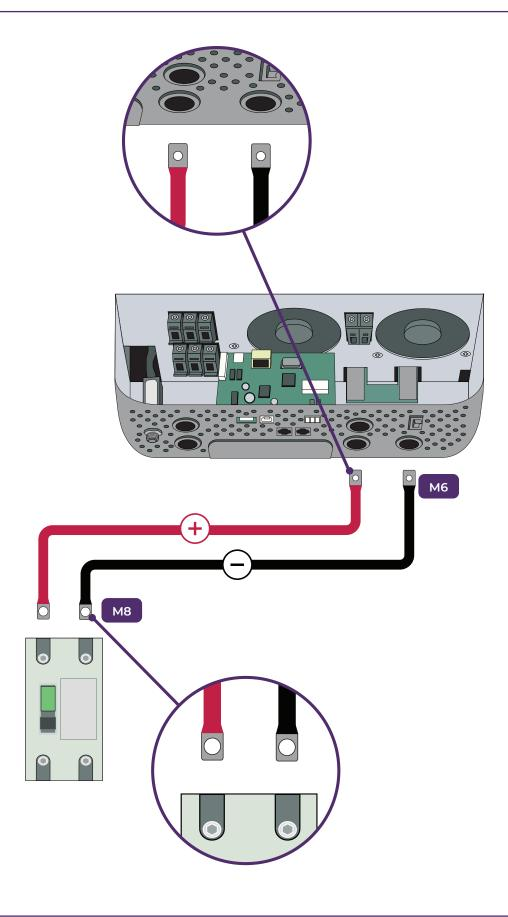
2 Before proceeding to connect the hybrid inverter to the 125A MCCB circuit breaker, align the 35mm<sup>2</sup> x 1m cables between the components to ensure that the M6 ends (smaller holes) are inserted into the hyrbid inverter, and the M8 ends (larger holes) are inserted into the circuit breaker.
