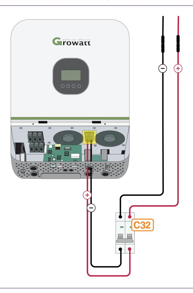
Run the excess 6mm² positive(+) and negative(-) cables from the C32 circuit breaker to the hybrid inverter.
