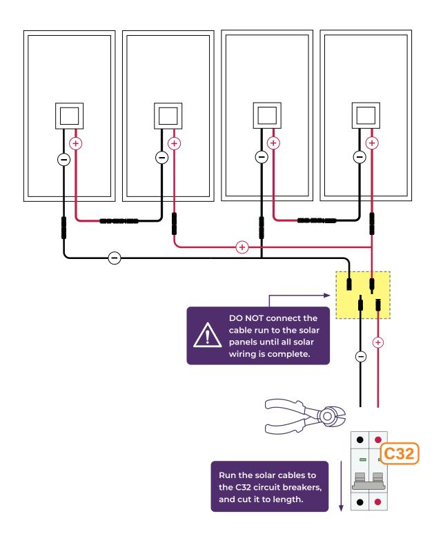
Run the 6mm² PV solar cables from the solar panels back to the C32 circuit breakers, and cuit it to length.
