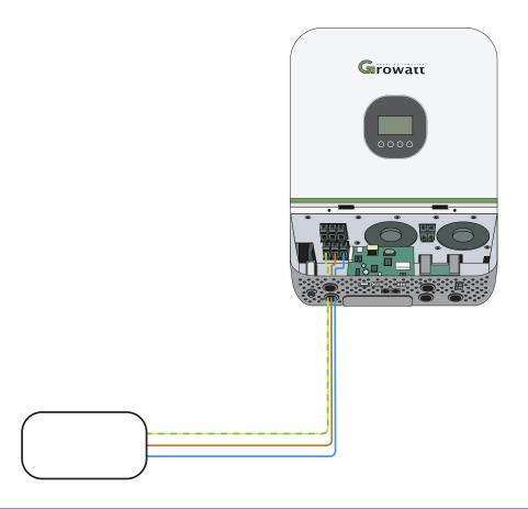
5 The output of the inverter is designed to wire into a distribution board.
