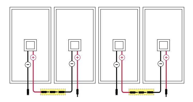
Start by creating two pairs of panels wired together. Connect the positive terminal of one panel to the inline fuse, then to the negative terminal of the next panel.
