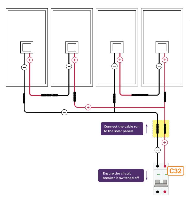
When the cables have been terminated in the circuit breaker and the circuit breaker is switched off, you can now connect the solar panels to the cable run. The circuit breaker must be switched off when connecting or disconnecting the solar panels from the cable run.
