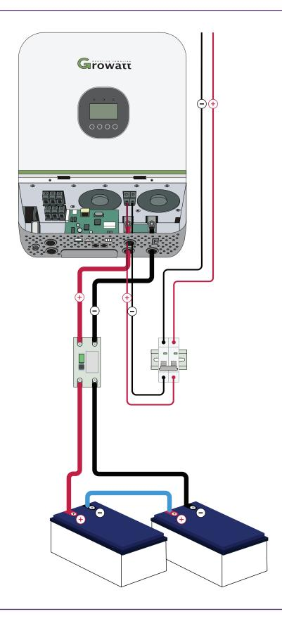
Once you have wired the batteries into the hybrid inverter, your completed wiring should look like the image above (excluding the panels). Double check everything is wired correctly and tightened before proceeding to prevent damage to your system.
