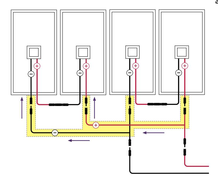
3 Connect the other pair of solar panels to the Y-branch connectors, connecting the negative terminals from each pair with the black Y-branch connector, and the positive terminals from each pair with the red.
