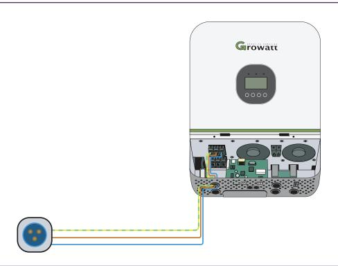
If using the utility / generator input, use components rated for 20A. If using components rated for less (e.g. a caravan plug), make sure to use an appropriately sized breaker.
