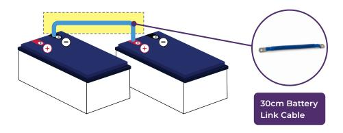
The battery bank is wired with two 12V batteries in series. This creates a 24V battery bank. The large gauge cable is used to connect the batteries together in series.
