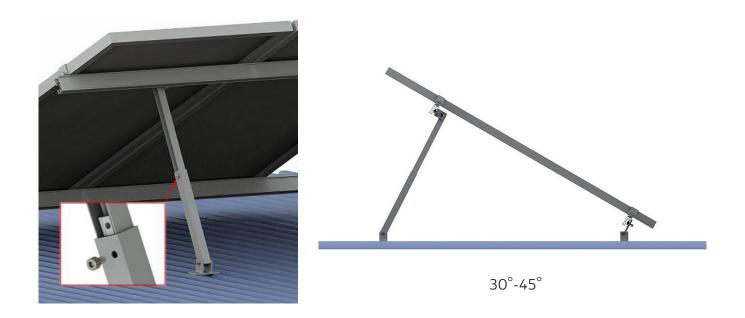
12 To adjust the angle of your tilt mount set up, loosen the bolt and adjust the angle to the desired degree, then tighten the bolt. The angle should sit around 30°- 45°.
