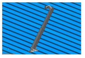
3 Attach the rear leg onto the roof using the roofing screws, ensuring the silicone pad is in place.
