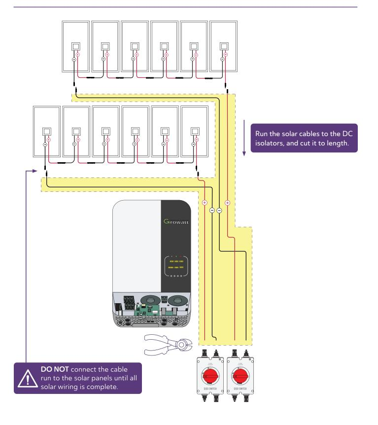
2 Run the 6mm<sup>2</sup> solar cables from the solar panels to the DC isolators, and cut it to length.
