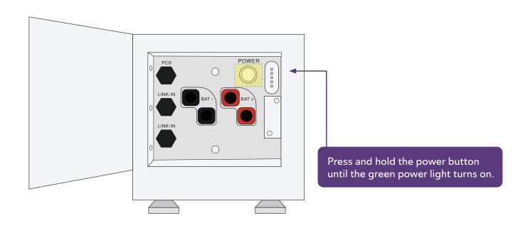
Power on all lithium batteries by pressing and holding the power button until the green light comes on.
