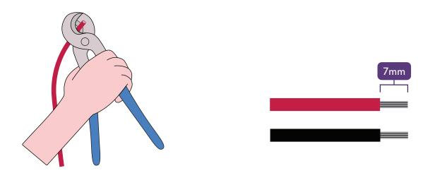
3 Use wire strippers to strip the ends off the black and red 6mm<sup>2</sup> solar cables. Strip the cables to approximately 7mm in length.
