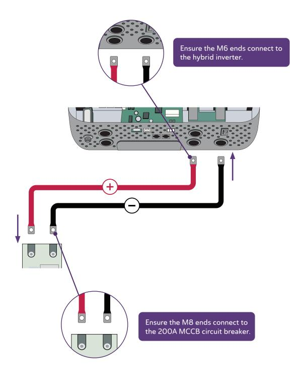
Before proceeding to connect the hybrid inverter to the 200A MCCB circuit breaker, align the 35mm<sup>2</sup> x 1m cables between the components to ensure that the M6 ends (smaller holes) are inserted into the hyrbid inverter and the M8 ends (larger holes) are inserted into the circuit breaker.
