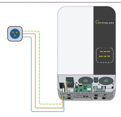
23 If using the utility / generator input, use AC cable rated for 40A. If using a plug, use a 32A rated plug.
