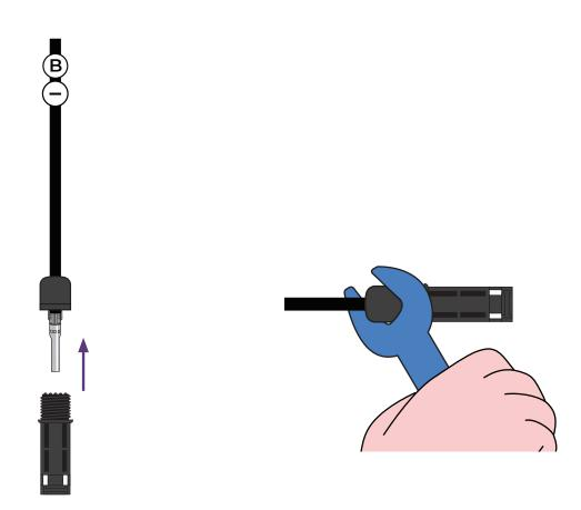
8 Insert the crimped "Metal conductor B" into the "Solar connector housing B" until it clicks, then tighten the gland nut using a spanner.
