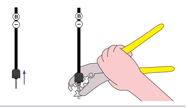
Move onto the black solar cable. Place the silicon gland and gland nut on to the cable. Crimp "Metal conductor B" onto the cable using the 4mm<sup>2</sup> crimping die.
