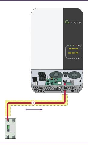
Wire the positive (+)  $35 \text{mm}^2 \times 1 \text{m}$  cable from the 200A MCCB circuit breaker to the hybrid inverter.
