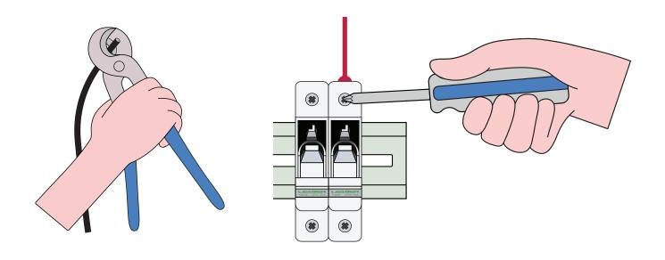
Ensure the fuse holders are disconnected by keeping them open with the fuses **OUT**. Use wire strippers to strip the ends of the solar cable, and terminate them in the fuse holders by inserting the stripped end and tightening the screw clockwise. Make sure the clamp inside the fuse holders are contacting the metal conductor, and **NOT** the insulation of the wire.
