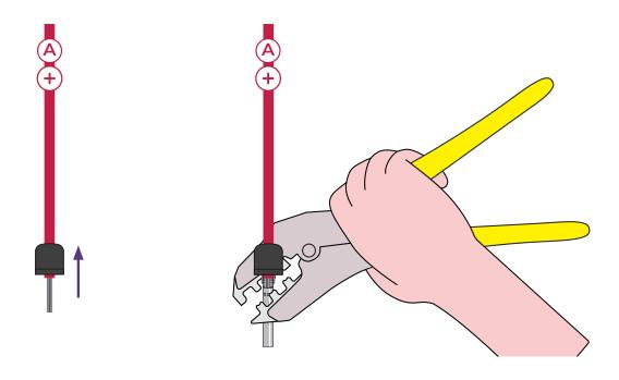
Starting with the red solar cable, place the silicon gland and gland nut onto the cable. Crimp "Metal Conductor A" onto the cable using the 4mm<sup>2</sup> crimping die.
