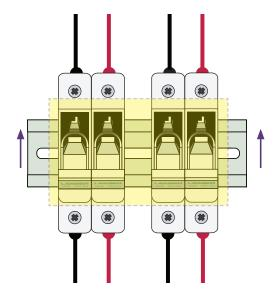
Then, connect the panels to the hybrid inverter by inserting the fuses into the fuse holder and closing the fuse holders.
