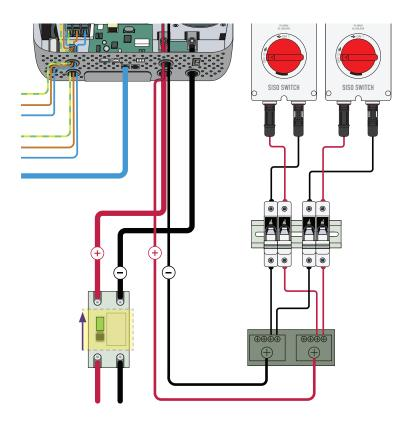
Switch on the circuit breaker and fuses in the following order. First, switch on the battery to hybrid inverter 200A MCCB circuit breaker.
