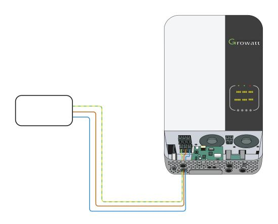
The hybrid inverter does not have an earth to neutral connection. This connection can be made at the main distribution board, unless the system is being used with a generator that also has an earth neutral connection.
