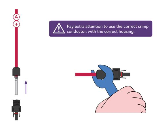
6 Insert the crimped "Metal conductor A" into the "Solar connector housing A" until it clicks, then tighten the gland nut using a spanner.
