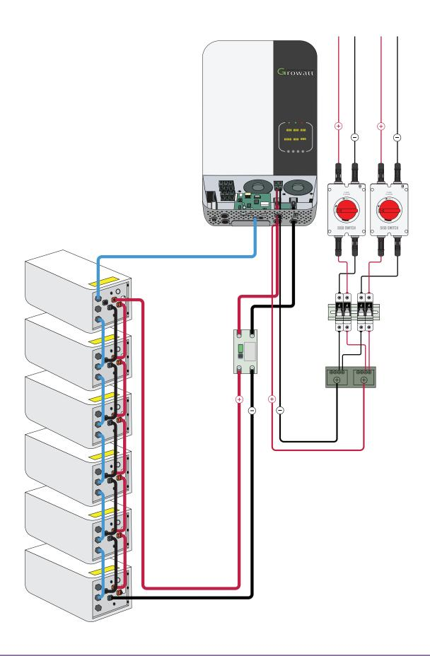
Once you've wired the batteries into the hybrid inverter, this is how the completed wiring should look (excluding the panels). Double check everything is wired correctly and tightened before proceeding, to prevent damage to your system. For this manual, all steps should be done by an electrician.
