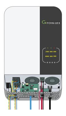
The Green LED on the PV Charge should flash, and the panel voltage should be around 200V-300V in full sunlight.
