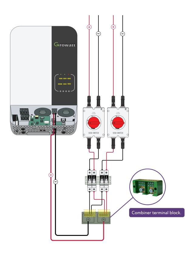
Use the green terminal combiner block to join both the negatives together in one side of the block, and both positives together in the other side. Then run the section of 16mm <sup>2</sup> cable from the M8 bolt terminals to the hybrid inverter.
