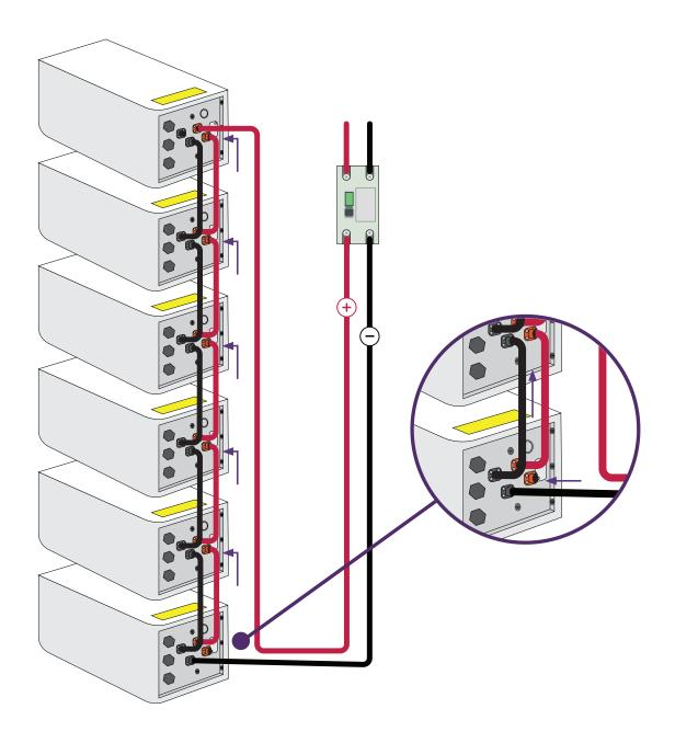
Connect the power connections, following the instructions detailed in the battery installation manual.
