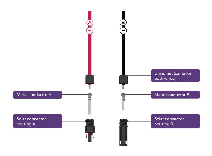
Ensure you use the correct metal crimp conductor, with the correct housing. Above demonstrates how each wire connects to its solar connector. The positive wire uses "Metal conductor A" and "Solar connector housing A", the negative wire uses "Metal conductor B" and "Solar connector housing B".
