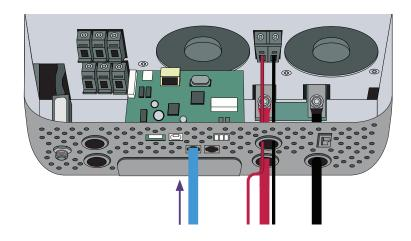
21 Connect the CAN communication cables as described in the battery installation manual.
