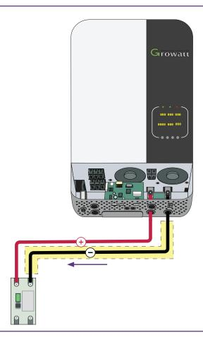
18 Wire the negative (-)  $35 \text{mm}^2 \times 1 \text{m}$  cable from the hybrid inverter to the 200A MCCB circuit breaker.
