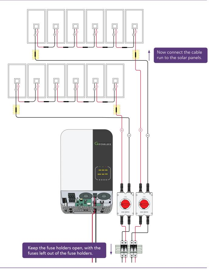
When the cables have been terminated in the fuse holders, with the fuses disconnected by keeping the fuse holders open with the fuses left out and the PV Array DC isolators switched "OFF", you can now connect the solar panels to the cable run. The fuses and DC isolators must be disconnected when connecting or disconnecting the solar panels from the cable run.
