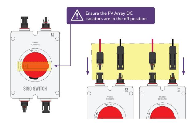
9 Ensure the PV Array DC isolators are in the off position. Then, connect the PV cable run from the solar panels. Ensure the other end of the cables stay disconnected from the solar panels.
