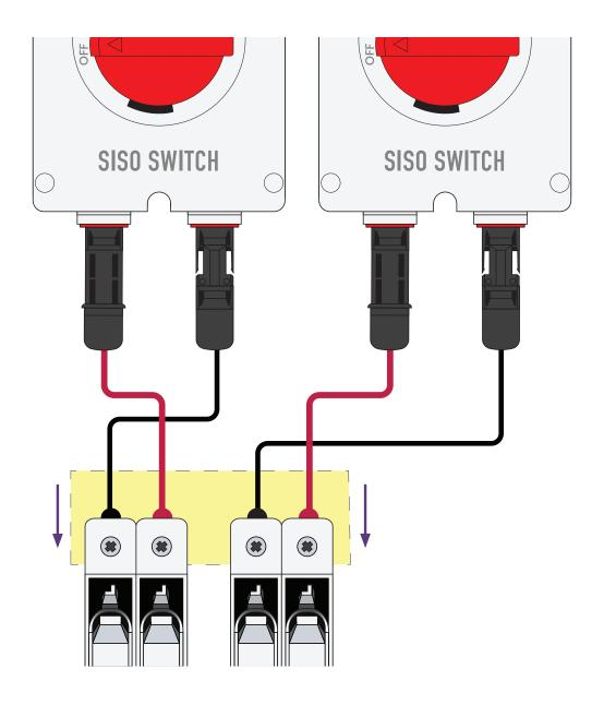
12 The PV Array DC isolators are now wired into the PV Array fuses.
