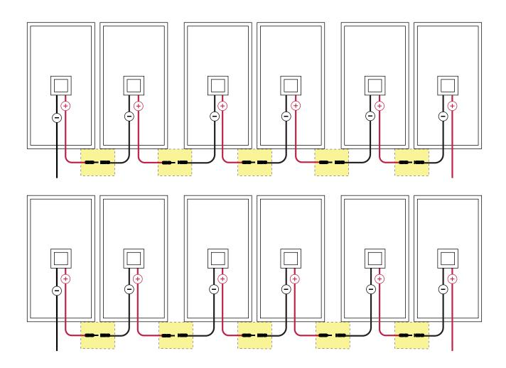
Start by creating two sets of six panels wired together. Connect the positive terminal of one panel to the negative terminal of the next panel for each string.
