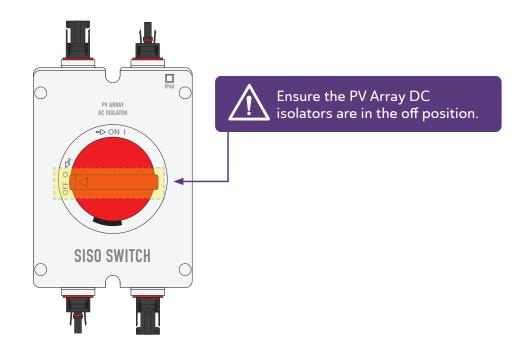
Ensure the 200A MCCB circuit breaker is switched "OFF" (switch in the down position, indicator showing green). Keep the fuses disconnected by ensuring the fuse holders are open with the fuses left out and the PV Array DC isolator is switched to the "OFF" position, before wiring.
