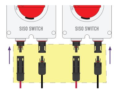
Repeat the process of crimping MC4 connectors onto a new set of cables (refer to page 9-11), which will connect the PV Array DC isolators to the PV Array fuses.
