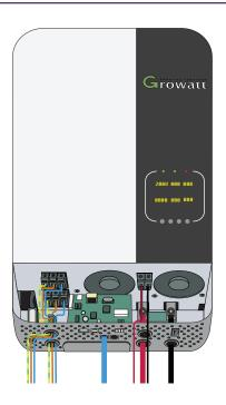
5 The green LED on the PV charge should be flashing, and the panel voltage should be around 180V-240V in full sunlight.
