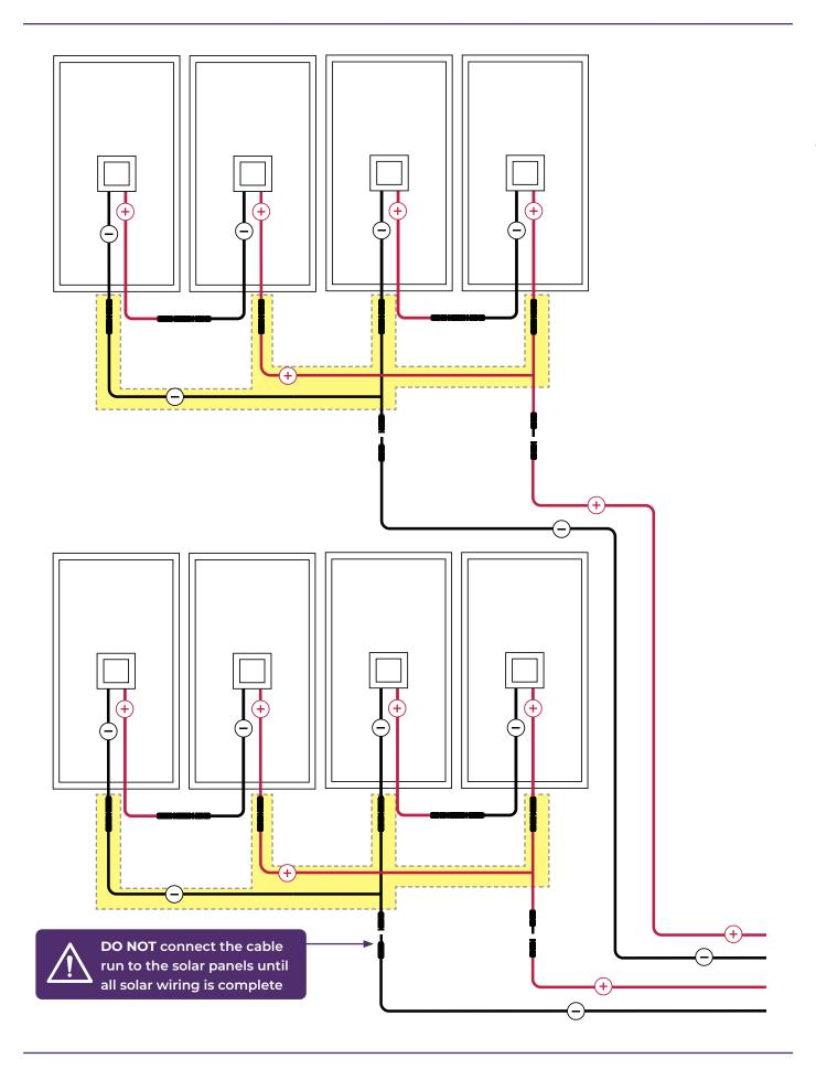
Connect the other two pairs of solar panels to the other set of Y branch connectors. This creates four outputs from the solar array: two positive(+), two negative(-).
