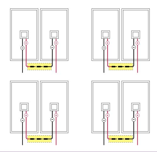
1 Start by creating four pairs of panels wired together. Connect the positive terminal of one panel to the inline fuse, then to the negative terminal of the next panel.
