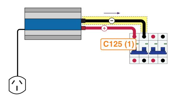
Wire the negative(-) 25mm<sup>2</sup> cable from the inverter to the C125(1) circuit breaker.
