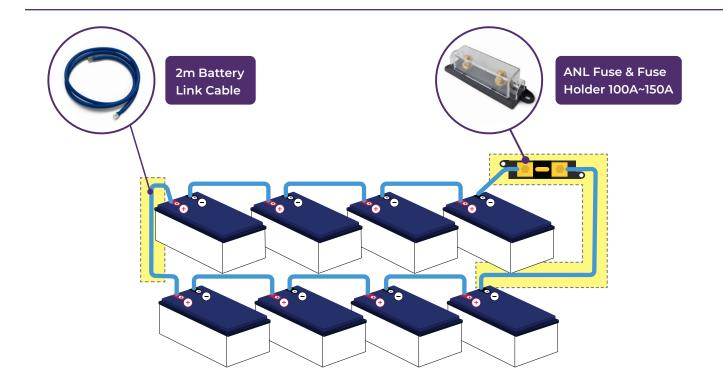
Wire a blue 30cm battery link from the **negative** terminal of the first row of batteries to the ANL fuse and fuse holder. Then, run one 2m battery link cable from the ANL fuse to the **negative** terminal of the second row of batteries. Lastly, wire the second 2m battery link cable from the **positive** terminal battery of the first row to the **positive** terminal battery of the second row.
