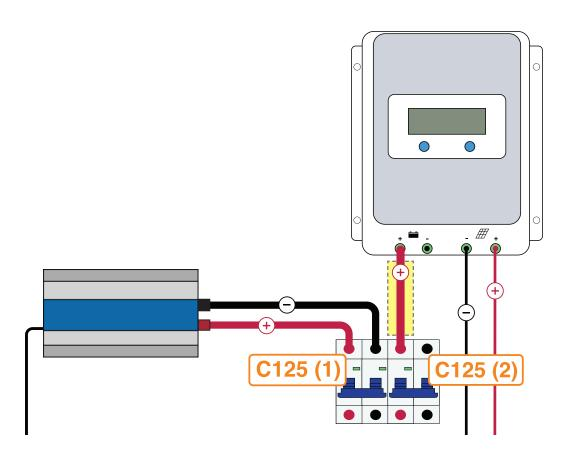
Wire the positive(+) 25mm<sup>2</sup> cable from the charge controller to the C125(2) circuit breaker.
