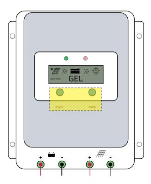
The system is now fully functional. The last step is to select the GEL battery charging mode on the charge controller. Click "SELECT" until the battery voltage interface is shown.
