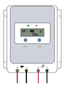
The green LED on the charge controller should be flashing, and the panel voltage should be around 60V-80V in full sunlight. As this charge controller auto-detects voltage, it can sometimes default to 12V on its first startup and give a battery over voltage warning.
