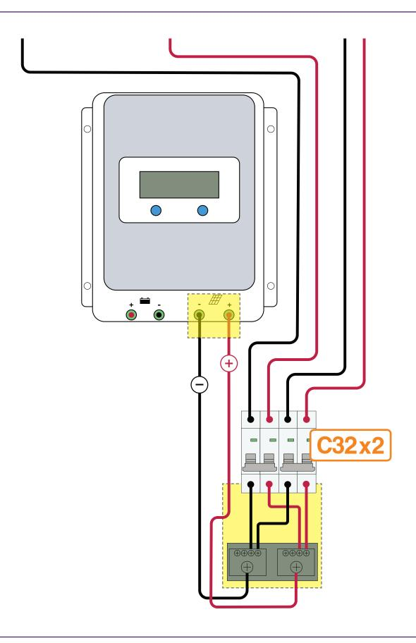
Use the green terminal combiner block to join both the negatives(-) together in one side of the block, and both positives(+) together in the other side. Then, run the section of 10mm <sup>2</sup> cables from the M8 bolt terminals to the inverter.
