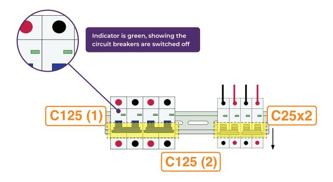
2 Ensure all circuit breakers are switched off before wiring (switch down, indicator showing green).
