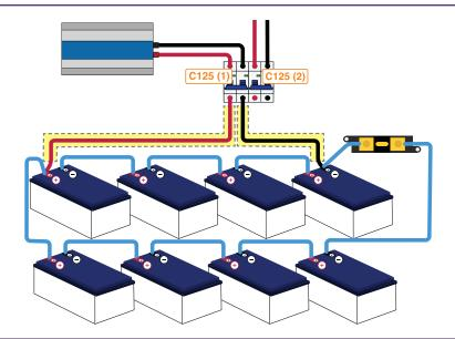
Wire one set of red and black 25mm<sup>2</sup> cable to the inverter through the C125 (1) circuit breaker.
