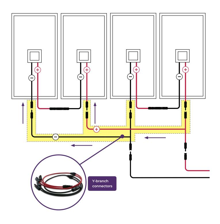
Connect one set of Y-branch connectors to two of the solar panel pairs, connecting the negative terminals from each pair with the black Y-branch connector and the positive terminals from each pair with the red.
