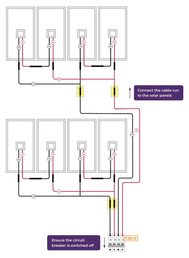
When the cables have been terminated in the circuit breaker and the circuit breaker is switched off, you can now connect the solar panels to the cable run. The circuit breaker must be switched off when connecting or disconnecting the solar panels from the cable run.
