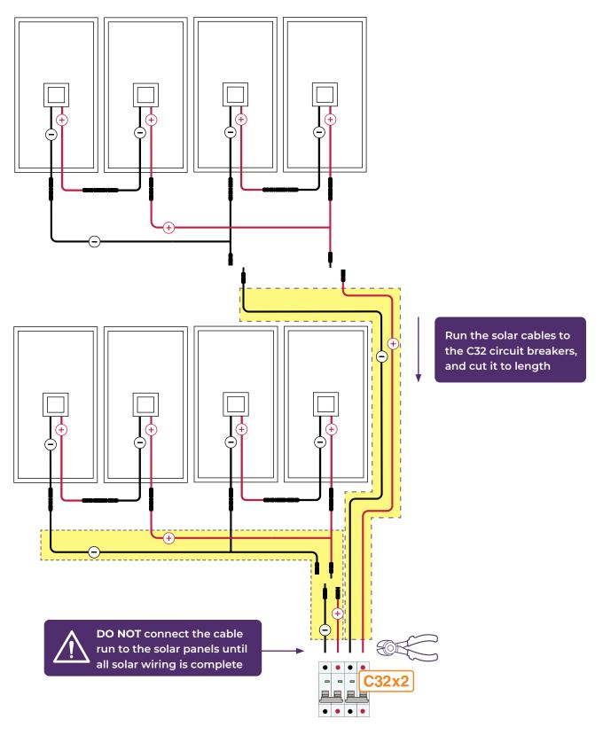
Run the 6mm<sup>2</sup> PV solar cables from the solar panels back to the C32 circuit breakers, and cut it to length.
