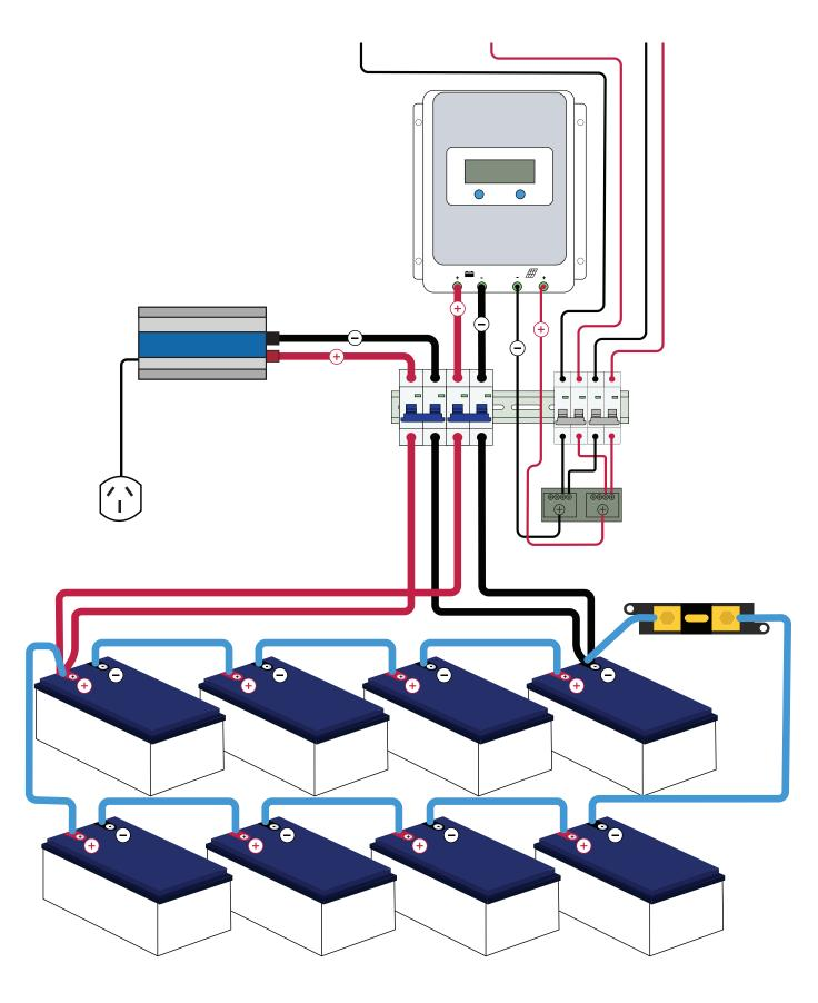
Once you have wired the batteries into the inverter and charge controller, your completed wiring should look like the image above (excluding the panels). Double check everything is wired correctly and tightened before proceeding to prevent damage to your system.
