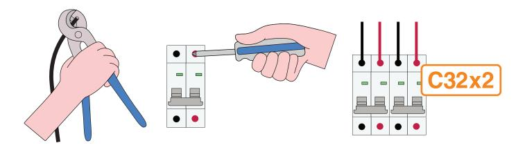
Use wire strippers to strip the ends of the solar cable, and terminate them in the circuit breaker by inserting the stripped end and tightening the screw clockwise. Make sure the clamp inside the circuit breaker is in contact with the metal conductor, and **NOT** the insulation of the wire.
