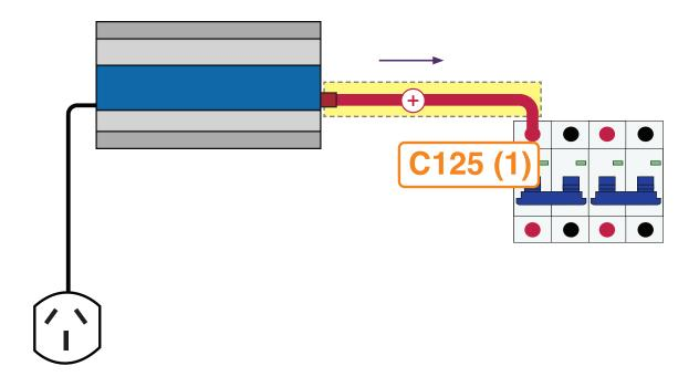
Wire the positive(+) 25mm² cable from the inverter to the C125(1) circuit breaker.
