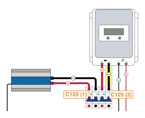
6 Wire the negative(-) 25mm² cable from the inverter to the C125(2) circuit breaker.
