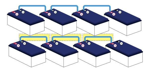
2 Wire the second row of four batteries together.
