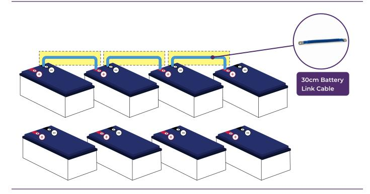
The battery bank will be wired with eight 12V batteries: two parallel sets of four in series to create a 48V battery bank. The large gauge cable is used to connect the batteries together and used to connect to the inverter.
