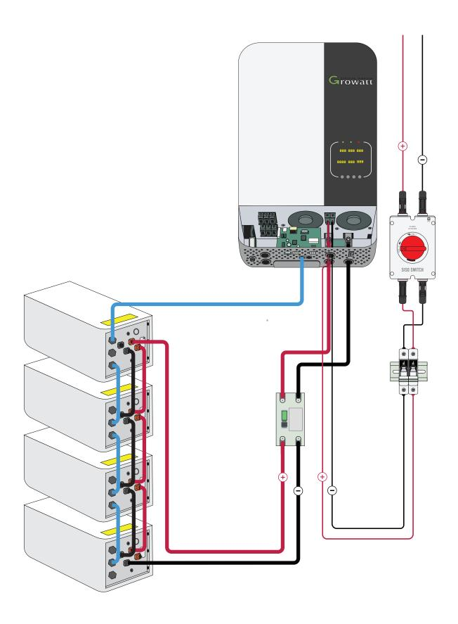
Once you've wired the batteries into the hybrid inverter, this is how the completed wiring should look (excluding the panels). Double check everything is wired correctly and tightened before proceeding, to prevent damage to your system. For this manual, all steps should be done by an electrician.
