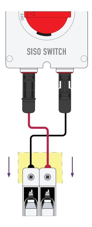
12 The PV Array DC isolator is now wired into the PV Array fuses.
