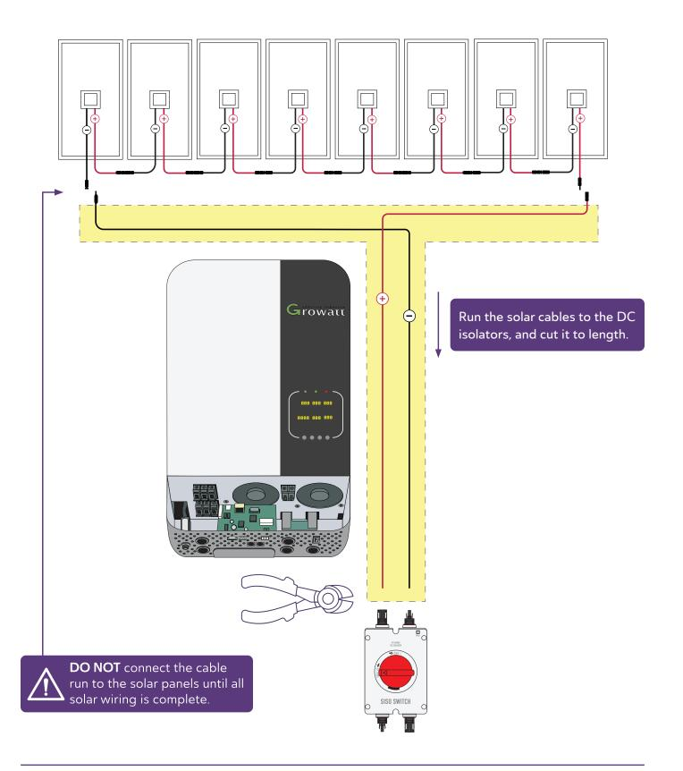
2 Run the 6mm<sup>2</sup> Solar Cables from the solar panels to the DC isolator, and cut it to length.
