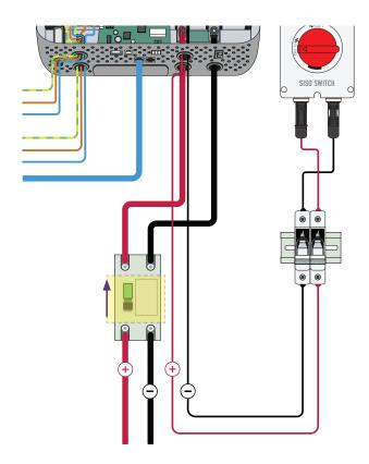
Switch on the circuit breaker and fuses in the following order. First, switch on the battery to hybrid inverter 200A MCCB circuit breaker.
