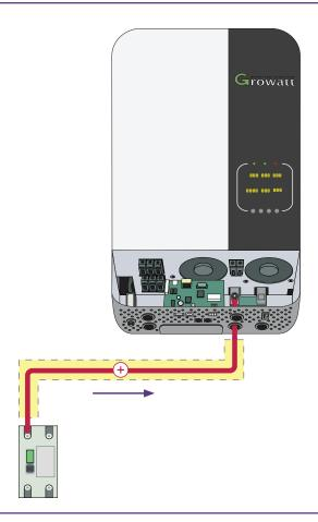
17 Wire the positive (+)  $35 \text{mm}^2 \times 1 \text{m}$  cable from the 200A MCCB circuit breaker to the hybrid inverter.
