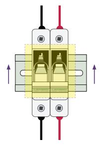
Then, connect the panels to the hybrid inverter by inserting the fuses into the fuse holder and closing the fuse holders.
