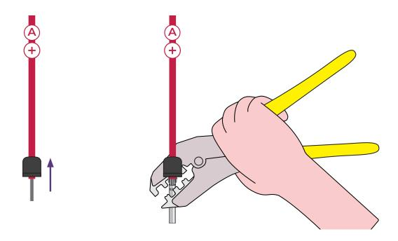
5 Starting with the red solar cable, place the silicon gland and gland nut onto the cable. Crimp "Metal Conductor A" onto the cable using the 4mm<sup>2</sup> crimping die.
