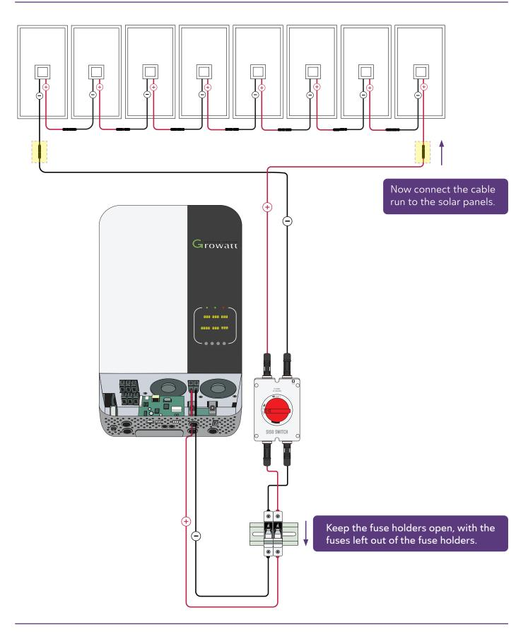
When the cables have been terminated in the fuse holders, with the fuses disconnected by keeping the fuse holders open with the fuses left out and the PV Array DC isolator switched "OFF", you can now connect the solar panels to the cable run. The fuses and DC isolator must be disconnected when connecting or disconnecting the solar panels from the cable run.
