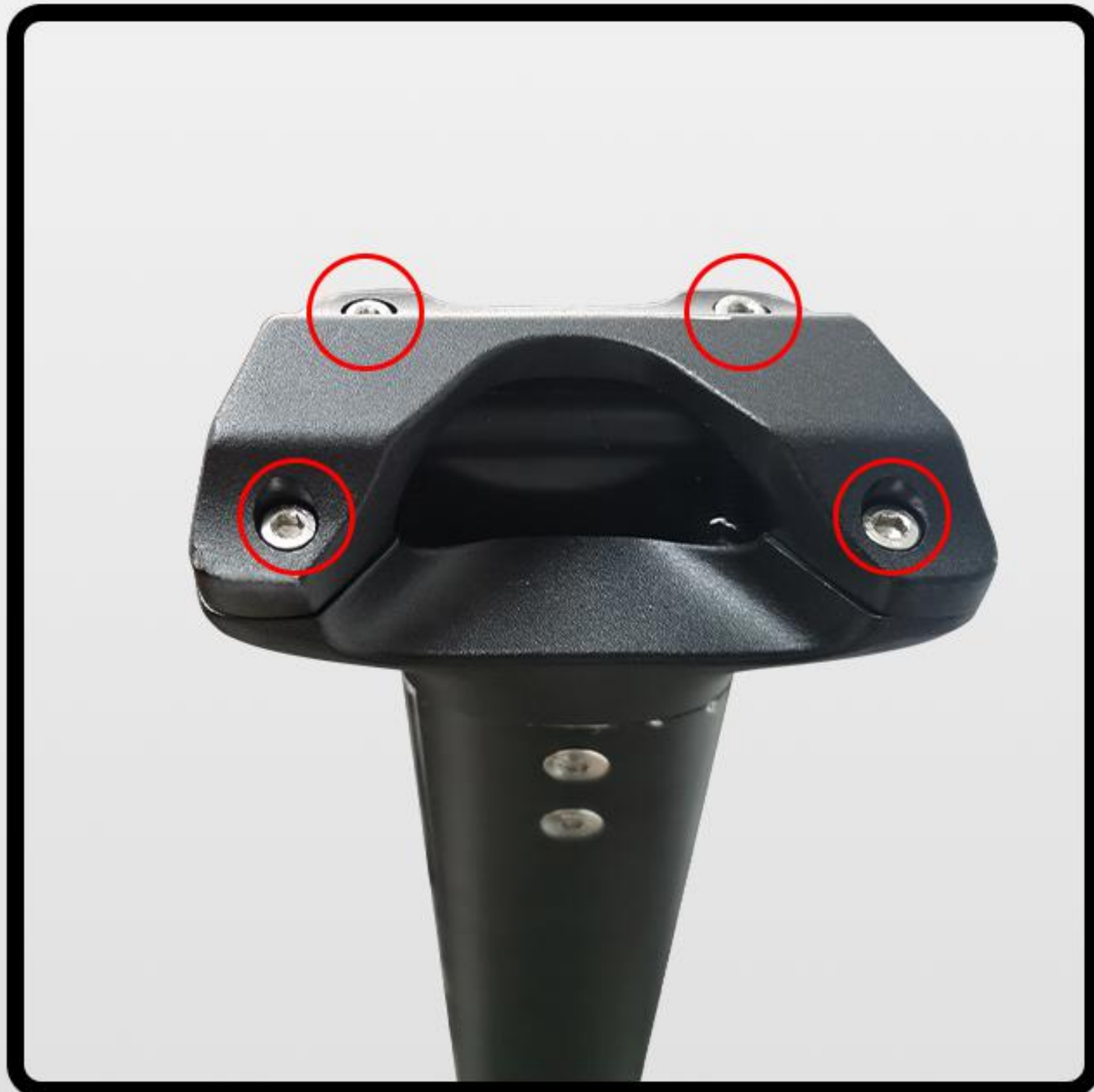
① Loosen the screws on the handle mount with a hex wrench, which is included in the basic tool kit.
