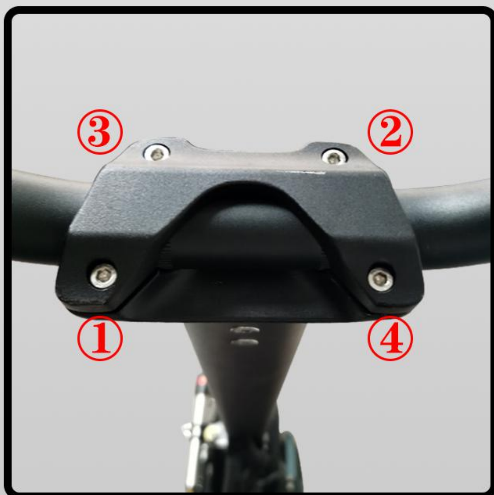
③ Progressively tighten the bolts in sequential order (1 to 4), ensuring equal tension balance between the mount and handlebar.
