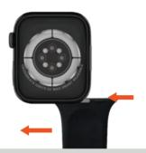
To attach the straps, slide in the bottom of the sharp into the gap on the watch case.
