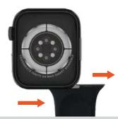
To remove the straps, slide the band outwards from the main watch casing.
