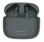
While charging – White light keep blinkingbased on the charge level Low Battery (less than 10%) – The first light will be on for 3 secs
