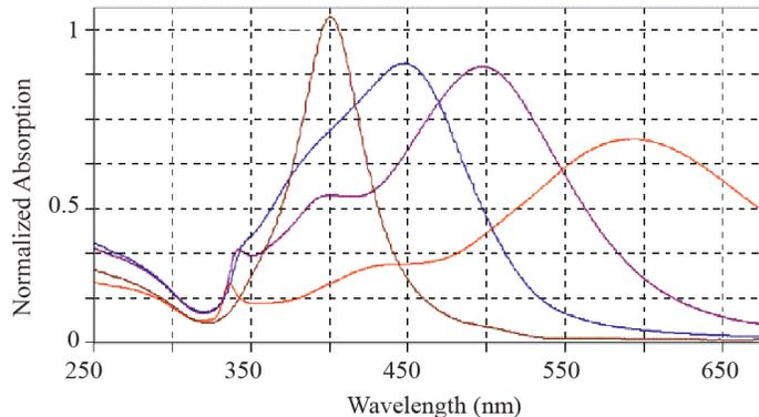
**Figure 2.** a) Optical images and the b) normalized absorption spectra of pentagonal silver nano-rods of various sizes.
