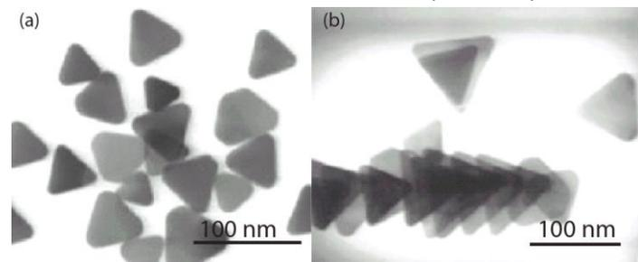
**Figure 1.** Scanning electron or Transmission electron microscopy micrographs of silver plates with average size of (a) 40±10 nm, (b) 50±10 nm.
