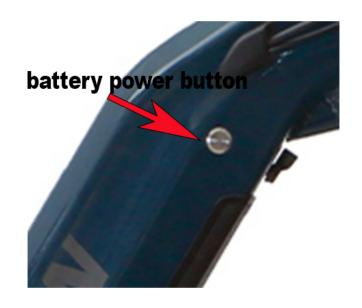
The instructions for the Ranger Power on/off are not as difficult as it may seem. To turn the Ranger Electric bike **ON** simply press the battery button on the right side of the frame for 0.05 secs (half a second) then turn on the display/controller power button immediately. If you looked at the battery out of its frame You can visibly see the power light illuminated when the battery indicator is pressed. If you do not turn on the display after engaging the power button the
