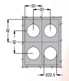
Minimum 30x40mm pitch between two actuators on a mounting surface. Minimum pitch between drilled holes for double and triple touch actuators is 30x55mm.
