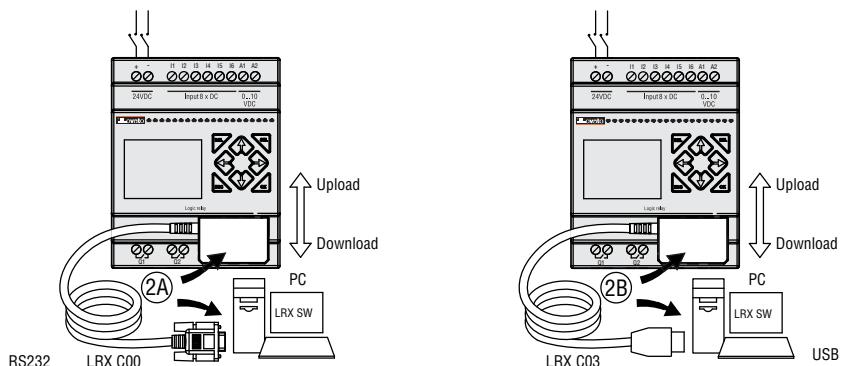
Connect the opposite end of the cable to the PC serial port on the computer depending on the connecting cable used.
