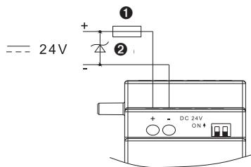
① - 1A fast acting fuse, circuit breaker and circuit protection.
