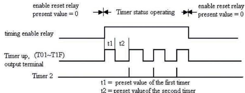
– The current value of Timer cannot be kept on a loss of power to LRD.
