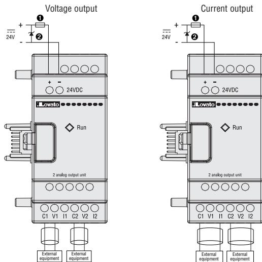
The output mode can be set by LRD... base module with DR register values (current mode):
