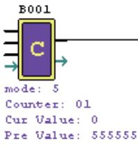
Note: Only first 31 Counter functions can keep their current value after a loss of power to the LRD.
