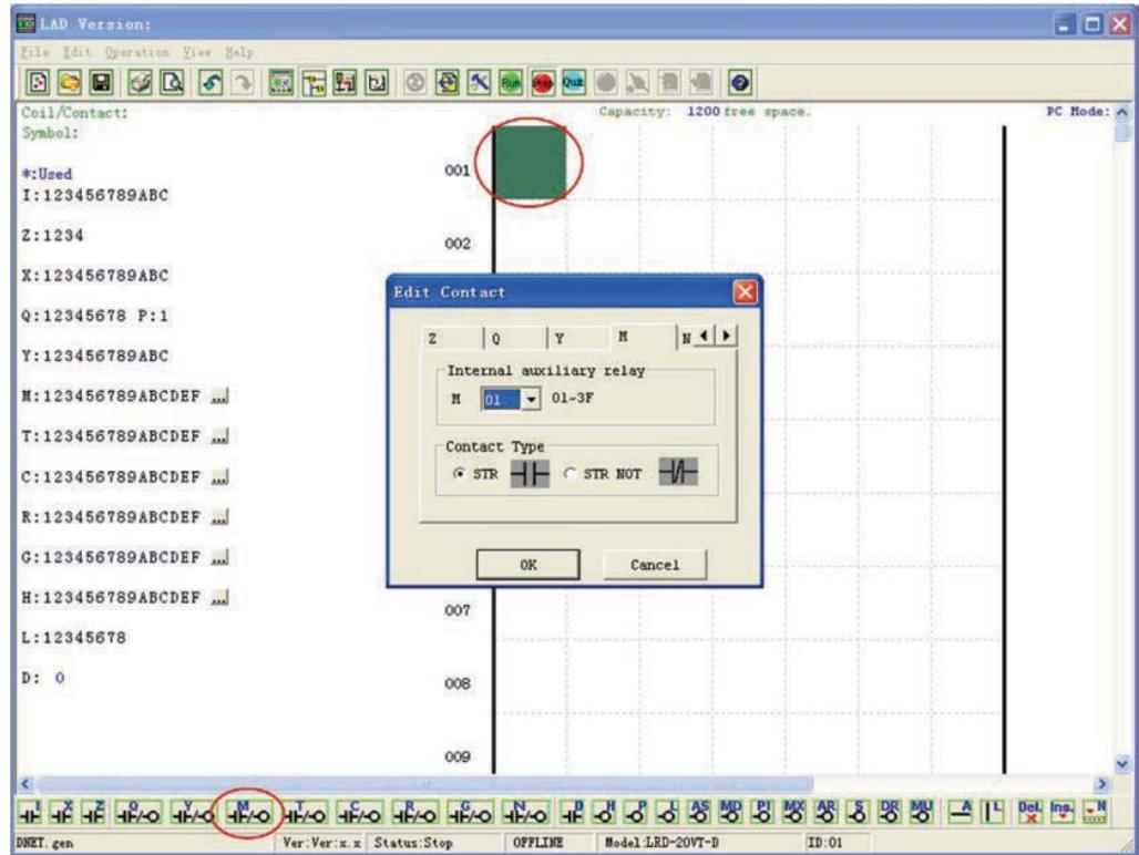
Note: If the ladder toolbar is not visible at the bottom of the screen, select View>>Ladder Toolbar from the menu to enable.
