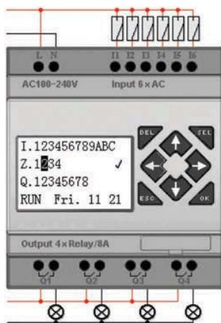
Press “ $\leftarrow$ ” to disable H03 coil, and the LCD display changes to initial frame.
