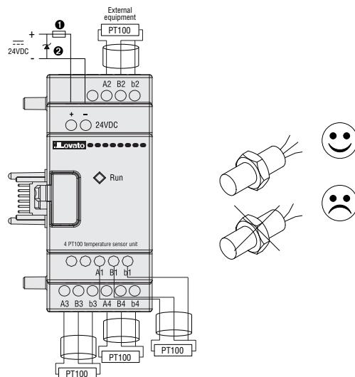
When the temperature is out of the -100°C...+600°C range limits, error output coils M34, M35, M36 and M37, which correspond to channel 1, channel 2, channel 3 and channel 4, will be activated (ON).
