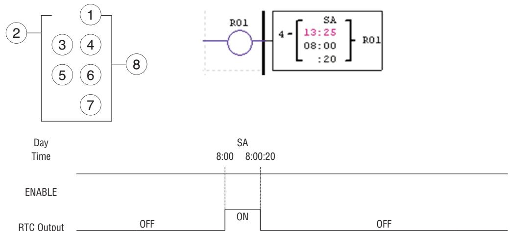
The present time will be 8:00:00 when it achieves 8:00:20 at first time, and RTC status bit R01 will be ON. RTC status bit R01 will be OFF when the present time achieves 8:00:20 at second time. Then time continuous going. So, this means that RTC status bit is ON for 21 seconds.
