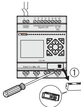
Insert the plastic connector end of the programming cable (LRXC00 for PC RS232 or LRXC03 for PC USB) into the LRD as shown in the figure below.
