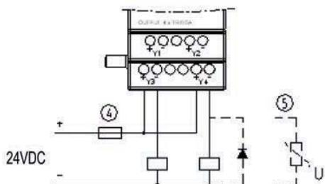
① 1A fast acting fuse, circuit-breaker or circuit protector.
