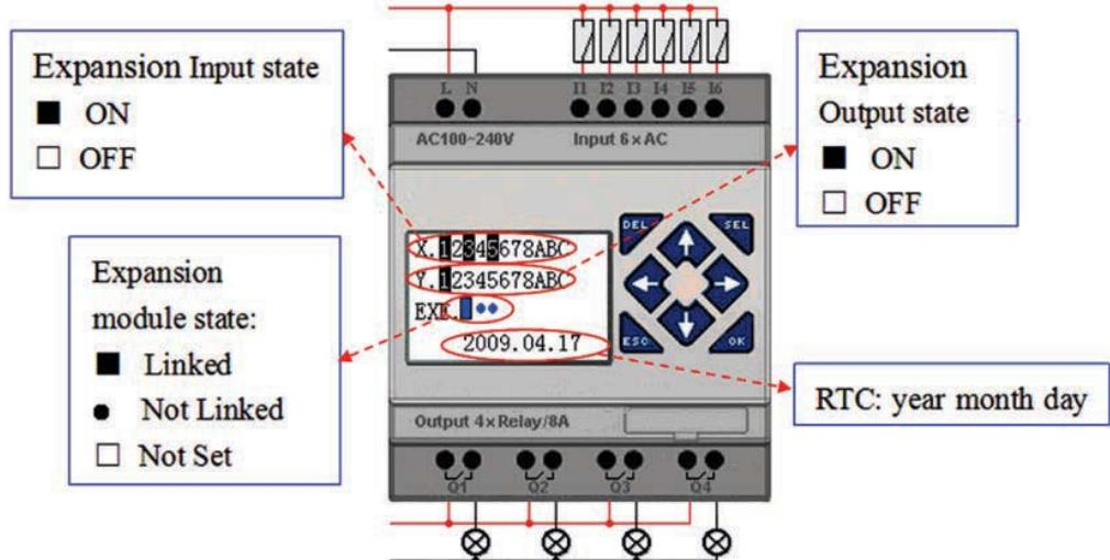
Digital IO module and Analog module both have indicator light. The state of indicator light is the same. The state of indicator light is shown below.
