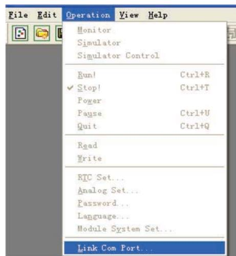
c. Select the correct Com Port number where the programming cable is connected to the computer then press the “Link” button.
