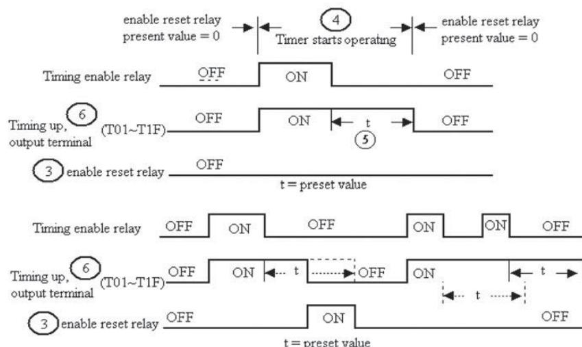
– TOE and TOF keep their current value after a loss of power to the LRD if "M Keep" is active, but the others' reset to 0.
