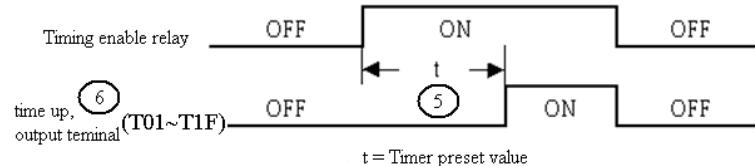
– TOE and TOF keep their current value after a loss of power to the LRD if "M Keep" is active, but the others' reset to 0.
