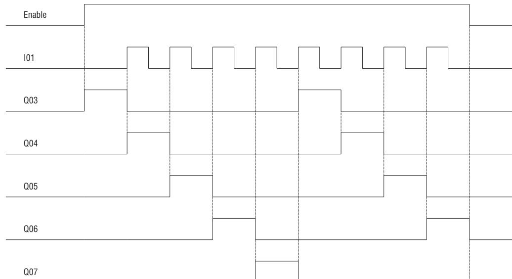
Q03 is ON, and from Q04 to Q07 are OFF when ENABLE is active. Q04 turns ON when I01 rising edge is coming on and other points turn OFF. The next coil turns ON at each rising edge of SHIFT input and others turn OFF.
