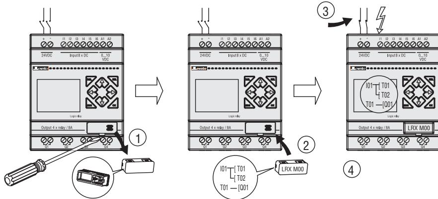
3. From the display keypad on the face of the LRD, select either WRITE or READ to transfer the program to LRMX00 or from the LRMX00 memory to the LRD.
