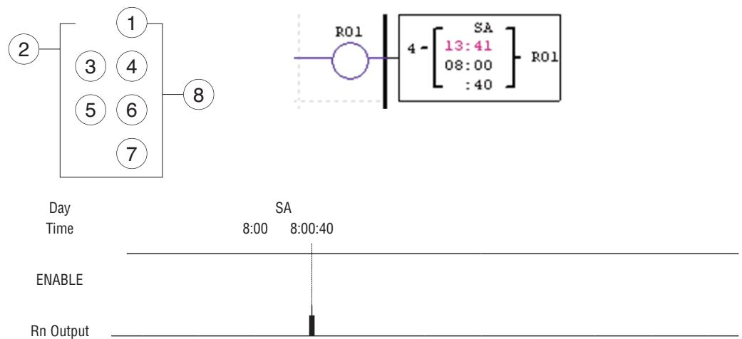
The present time will change to be 8:01:00 when it achieves 8:00:40, and RTC status bit R01 turns ON. Then time is ongoing on and R01 turns OFF. This means that the RTC status bit will be ON for one pulse.
