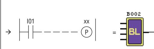
Note: The input terminal is NOP which is equivalent to "Low".
