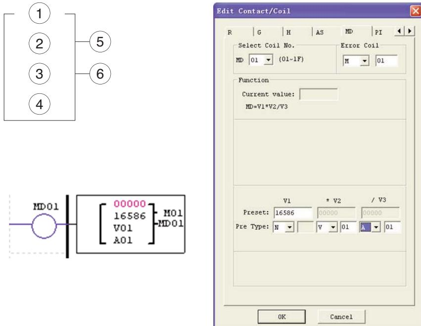
Error output coil M01 will turn ON when the compute result is overflow.
