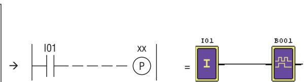
Note: The input terminal is NOP which is equivalent to "Low".
