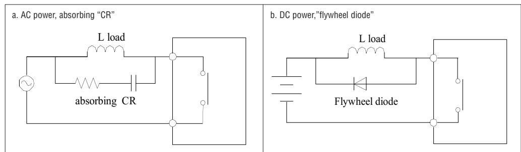
Do not use capacitance alone as absorbing as shown below.
