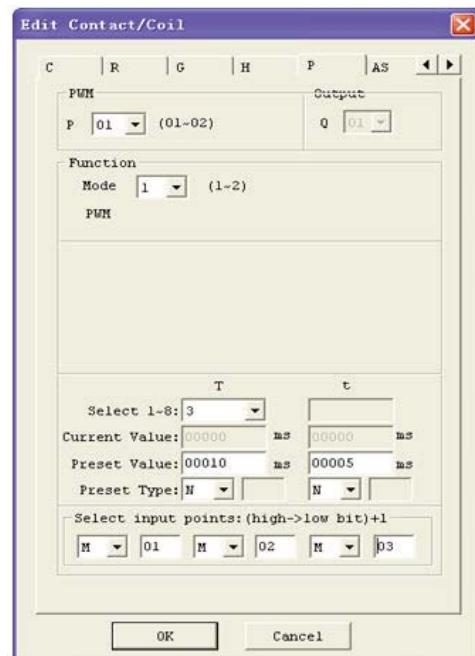
The state of M01, M02 and M03 are 010, so PWM output pulse is like this setting below:
