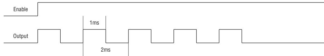
PLSY stops outputting when the number of output pulse is completed.
