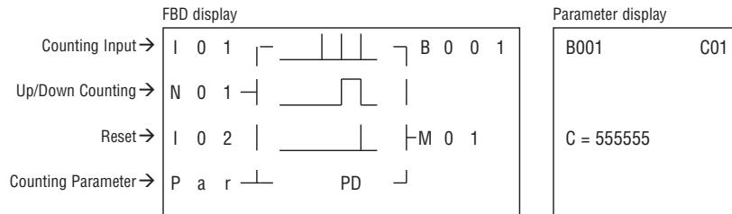
Note: The "PD" means the current value will be retained until the power recovers; Counter keeps current value when the LRD switches between RUN and STOP when C KEEP enable.
