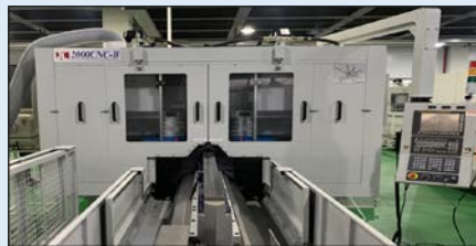
Grinding of the block and rails
