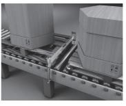
Reliable detection of different objects and objects with cutouts and openings, here pallets:
