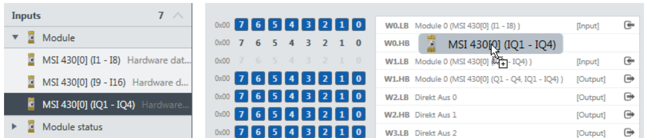
Fig. 8.24: Adding of bytes to the gateway process image (T→O) using drag-and-drop in MSI.designer
