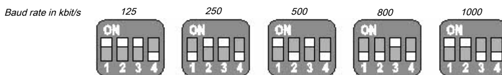
Fig. 10.2: Setting the DIP switches on the MSI-FB-CANOPEN module
