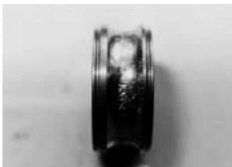
Fig. 15-1 Generation of Flaking on Inner Ring Raceway of Deep Groove Ball Bearing
