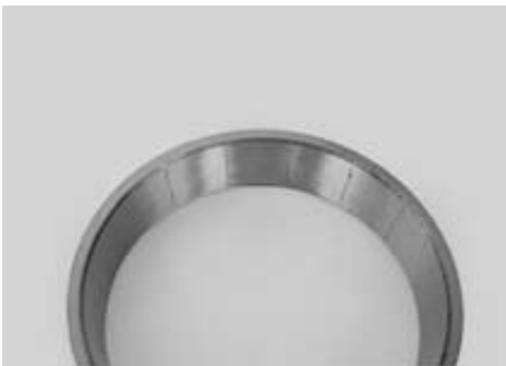
Fig. 15-7 Indentation Marks on Outer Ring Raceway of Tapered Roller Bearing
