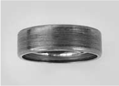
Fig. 15-9 Creep on Outer Ring Surface of Deep Groove Ball Bearing
