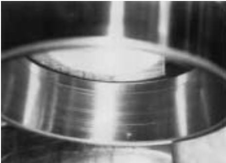
Fig. 15-3 Scratches on Outer Ring Raceway of Tapered Roller Bearing
