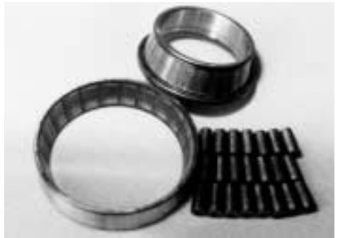
Fig. 15-12 Corrosion on Tapered Roller Bearing
