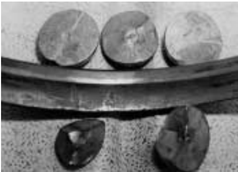
Fig. 15-5 Crack on Outer Ring Raceway of Deep Groove Ball Bearing
