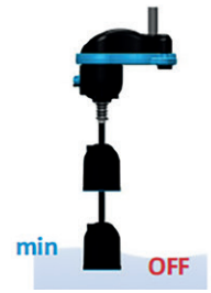
Low level stops the pump
