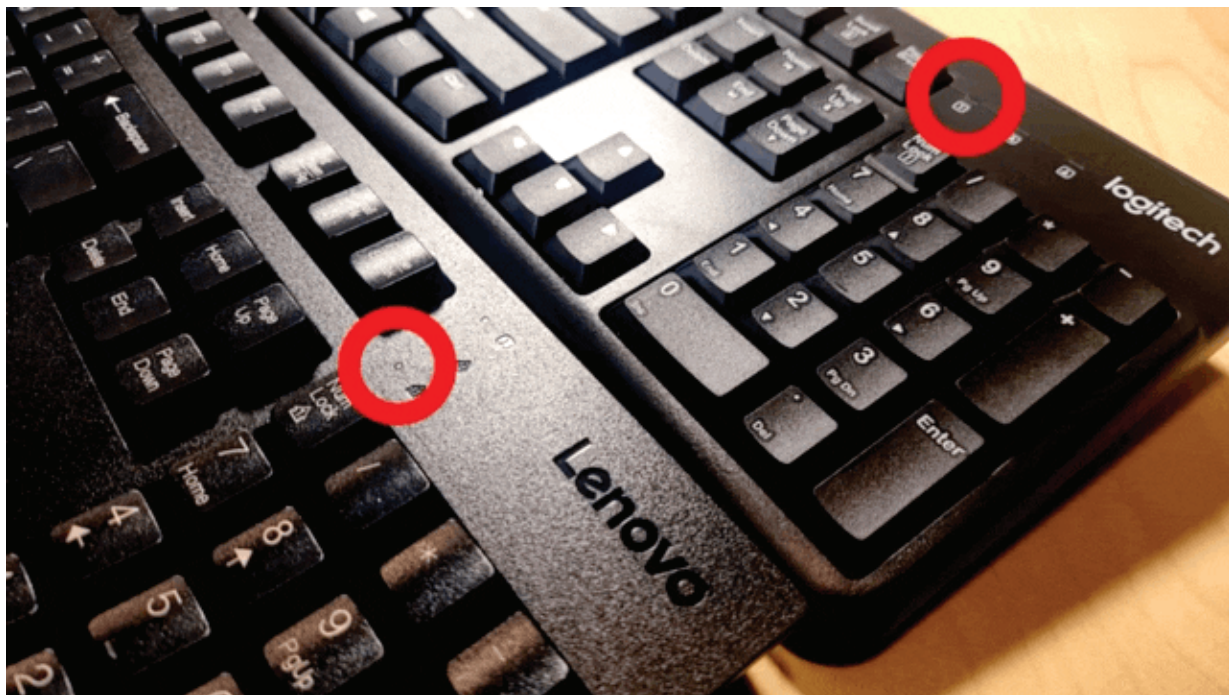
With both keyboard attached to a modern PC, pressing the caps lock key on the Lenovo keyboard with light both Lenovo and Logitech keyboards caps lock LED.
