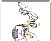
3) Turn the knob horizontally to unlock (3) and peel off the protective film from the suction pad (4). Position the mounting bracket on the windshield and press tightly to secure position. Once positioned, turn the knob vertically to lock in place(5).
