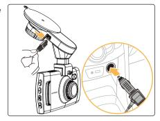
6) Turn on the engine. The dash camera will power on and start recording. Video files are stored on the memory card. When the memory card fills up, the newest video files will start to replace the oldest video files (called loop recording) – so you will always have the most recent video files.
