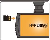
Gently slide the dash camera along the connector on the mounting bracket(1). Then, carefully remove the protective film from the lens (2).
