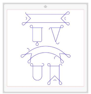
When a design is intricate or small and round, Silhouette Studio<sup>®</sup> will put in the appropriate loops and hooks to orient the Rotary Blade, but that may not be enough to orient the blade correctly. That is why we have created the following guidelines.
