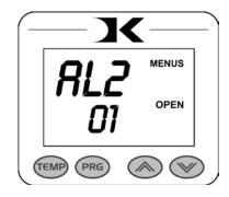
displays. The PPR menu must be set to ON for this menu to be visible. Use the arrow keys to set AL2 to OFF, or 1 through 10.
