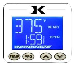
depending on if it is cooling down or heating up to the set temperature. READY is shown only if the current temperature is within 5 degrees of the set point temperature.
