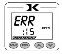
Once the temperature signal is restored (no longer broken, or plugged back into the control) the press will resume the temperature display, and start heating if necessary. If ERR persists, contact support.
