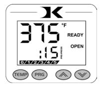
the main timer for 20. When the operator activates the press, the 5-sec time counts down. When the press releases, the time setting switches to 20 seconds.
