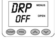
If the current temperature drops below the set temperature by that many degrees, and alarm will sound. Press TEMP to silence the alarm.
