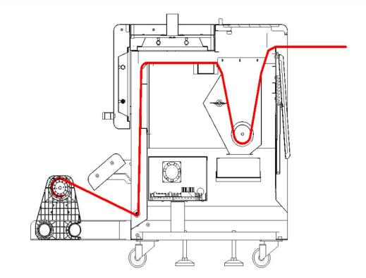
**4.1.** Lead the media into powder box, though outside powder bar, then cross the space between up dryer and platform dryer, wind the media to the paper tube of the take up winder, the winding operation complete.
