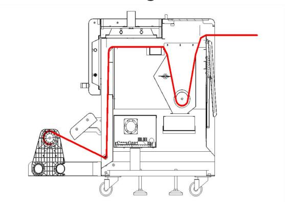
**4.1.** Lead the media into powder box, though outside powder bar, then cross the space between up dryer and platform dryer, wind the media to the paper tube of the take up winder, the winding operation complete.
