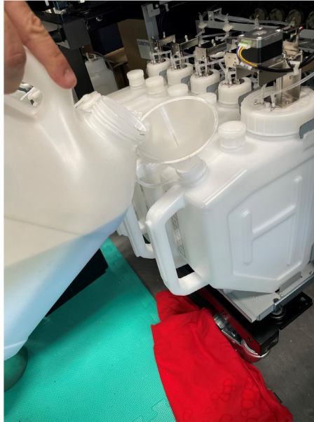
Figure 5. Adding ink to the main tank.
