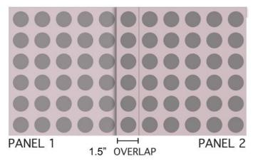
2 CUT THROUGH THE CENTER OF THE OVERLAP AREA FROM TOP TO BOTTOM USING A STRAIGHT EDGE AND A SHARP BLADE REMOVE TRIM FROM PANEL 2
