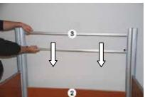
Make sure all panels are pushed all the way down. Slide raceway-frame 3 on top of half-panel 2.
