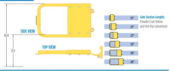
**Self-Closing Gate:** Approved product: GuardDog Self-Closing Safety Gate: Provide maximum opening coverage when used with OSHA compliant guard rails
