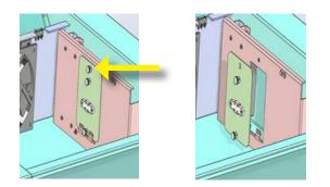
2. Remove the Bracket Assembly by unscrewing the top thumb screw.
