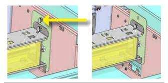
2. Remove the Bracket Assembly by unscrewing the top thumb screw.
