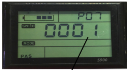
One magnet for speed sensor
