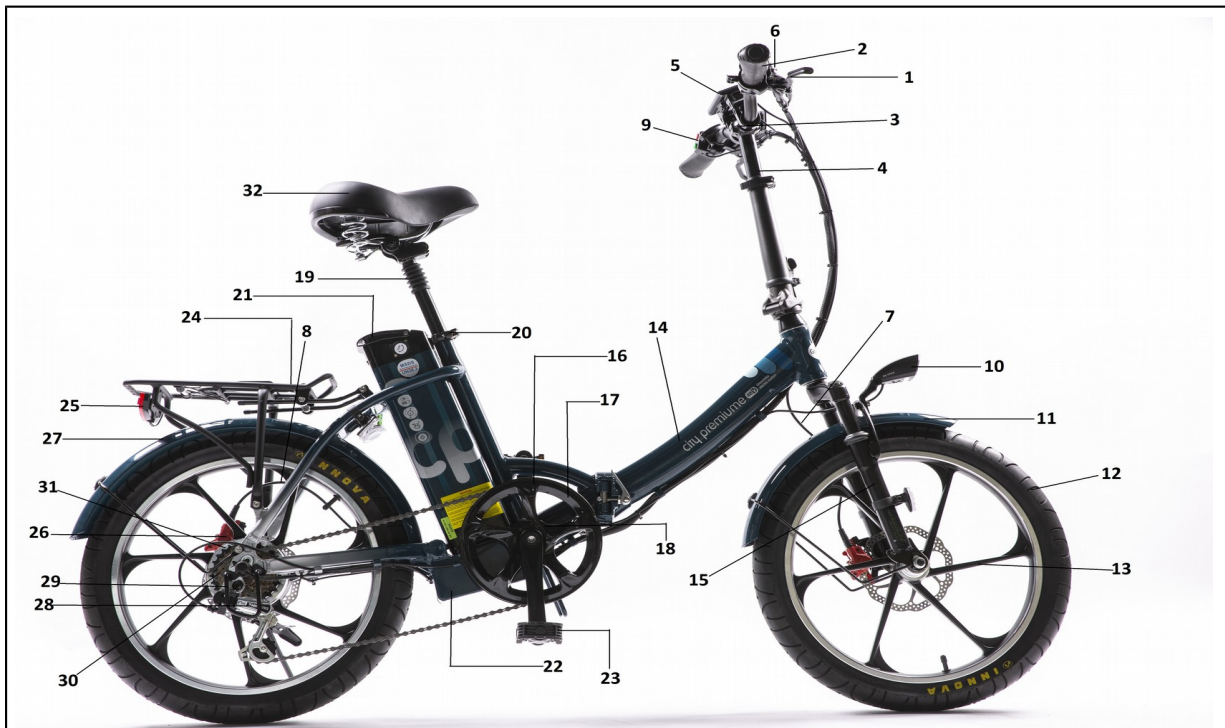
1-Brake Handles. 2-Grips. 3-Handlebars. 4-Adjustable Stem. 5-Display. 6-Gear Shifter. 7-Front Brake Cable. 8-Rear Brake Cable. 9-Head light and horn. 10-Front Light. 11-Fender. 12-Tire and Inner tube. 13-Front Wheel. 14-Frame. 15-Front fork. 16-Front wheel gear (Crank). 17-Chain shield. 18-Pedal assist sensor. 19-Shock absorber for seat. 20-Seat Clamp. 21-Lithium battery. 22-Motor Controller. 23-Pedal. 24-Rear Rack. 25-Rear Light. 26-Rear Brake. 27-Rear Fender. 28-Derailleur. 29-Mechanism protection. 30-Gears. 31-Motor. 32-Seat.
