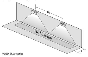
Using multiple units mounted at a typical 7.5' delivers 14' center-to-center spacing on a 6' wide egress path.
