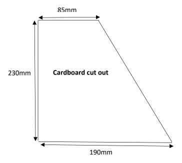
After its been cut out take this template and fit it into your bicycles frame as illustrated below be sure to keep the bottom section at 180 degrees (straight line)
