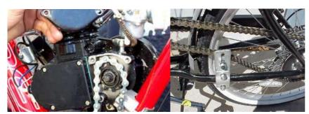
**Cut chain to length and using master link put chain back together.** Do not cut chain too short! Install idler pulley. Do not over tighten chain. Install chain guard. Use some tin snips to cut cover at the rear if needed. Use a good zip tie at the rear and the extra long bolt for the counter shaft cover will hold the front
