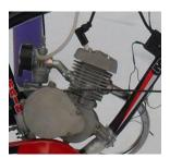
The engine is designed to fit between the down tube and the seat tube of a standard frame bicycle. Other types of bicycle may require slight modifications
