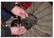
4) Thread the nine bolts through the sprocket and use the half moonmbacking plates on the inside. Mount the sprocket to the rear wheel as shown. Do not over-tighten and make sure that the sprocket is exactly perpendicular to the axis of the wheel. Reinstall the rear wheel to bicycle
