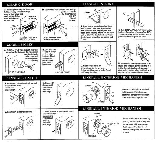
Suitable for door thickness: 1-3/8"(35mm) to 1-3/4"(45mm)
