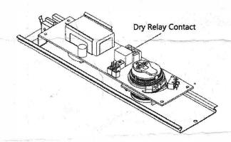
B- Use Dry Relay Contact shown in diagram to connect Alarm Unit to a magnet or strike as desired. For a more audible or visual alarm, a DC horn or light could be used in place of magnet or strike. See step 3 for different wiring diagrams.
