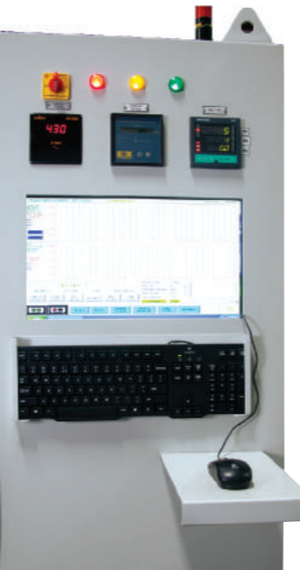
PLC BASED SHEET THICKNESS MEASUREMENT & CONTROL
