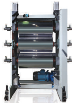
CALENDAR ROLL SIZE Roll Dia. (mm): 310, 350, 400 Roll Width (mm): 650, 800
