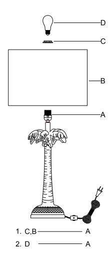
110-120V / 60Hz E26 MAX 60W TYPE A (Do not contain light bulb)
