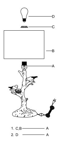
110-120V / 60Hz E26 MAX 60W TYPE A (Do not contain light bulb)
