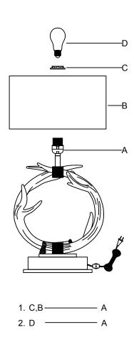
110-120V / 60Hz E26 MAX 60W TYPE A (Do not contain light bulb)
