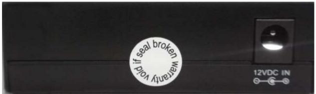
The DC Jack on the rear panel can be connected to power supply adaptor with the DC input.
