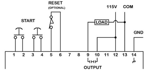
**MAINTAINED OUTPUT** - An optional Hold switch can be wired into the circuit of the 4480 to provide a maintained output. When the Hold switch is closed, the load will stay energized even after the start switches are released. The Hold switch must not close until the pinch-point is passed, and should remain closed for the rest of the machine cycle.
