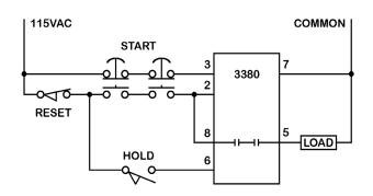
Note: The Reset and Hold switches shown in the above wiring diagrams are optional and are not required for all applications.
