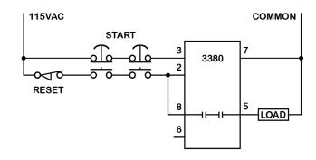
MAINTAINED OUTPUT: In order for a machine cycle to begin, both start switches must be pressed within .5 sec. (this time is internally adjustable). The output will remain energized as long as the start switches are depressed.
