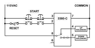
Note: The Reset and Hold switches shown in the above wiring diagrams are optional and are not required for all applications.
