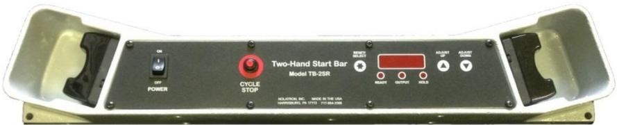
The Start Bar is an ergonomic starting system used to reduce operator stress that can lead to carpal-tunnel syndrome. An internal anti-tiedown control monitors both start sensors for concurrent operation. The output utilizes redundant positive guided relays which are monitored to ensure proper operation.
